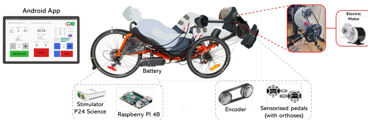
148 Figure 1: FES-Bike prototype. A commercially available trike (Catrike 700) with an absolute magnetic encoder (AS5047P, ams 149 OSRAM) and sensorised pedals on the crank side. Behind the seat, there is a battery, as well as a box containing a Raspberry Pi 150 4B, a neurostimulator (P24 Science, Hasomed) and other electronics. Highlights in red show a detail of the motor mounted on 151 the trike frame and coupled with a second transmission chain, enabling assisted pedalling and moving the passive legs. This 152 element of the setup was then removed for the race. On the left a detail of the main page of the Android control application. 153 The figure is composed using BioRender.com.
